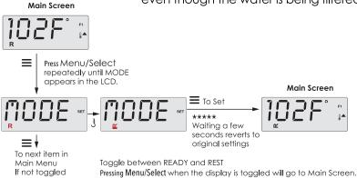
READY Mode will allow the spa to Poll and determine a need for heat. The panel will maintain a "current" temperature display.
